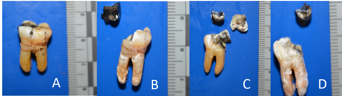
FIG. 1 – Example of Watchdog® Battery Acid effects on silver amalgam samples. A) Before exposure, score=0; B) After 2-hours exposure, score=3 (note separation of restoration); C) After 72-hours exposure, score=3; D) After 120-hours exposure, score=3 (note chalky appearance).
