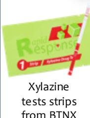
Six synthetic urine samples spiked with xylazine standards at different conc. and 36 human urine samples were tested to evaluate strip sensitivity and specificity. Quantitative data was obtained from an in-house GC-MS method for xylazine. Urine samples were tested within 1-13 days after collection and kept at 5 °C until analyzed.
