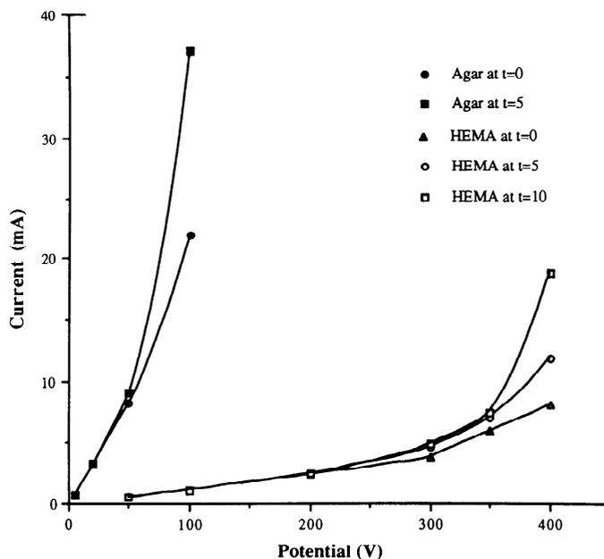
FIG. 1. Representative current vs. voltage curves for 12-cm-long salt bridges composed of 0.15 M NaCl and either agar or poly-HEMA as described in text. Each data point represents average of 3 measurements on 5 equivalent bridges. Change in conductivity secondary to joule heating is indicated by increasing steepness of slope of curves with increasing time of power dissipation.  $t = 0$ , Initial time of power dissipation;  $t = 5$  and 10, 5 and 10 min after power dissipation, respectively.
