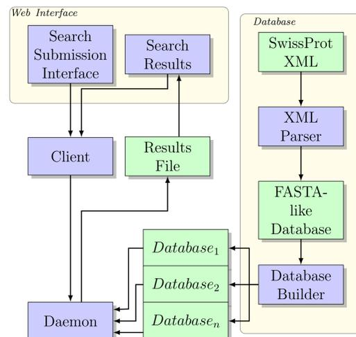
Figure 1. Diagram of the BUPID Top-Down system.
