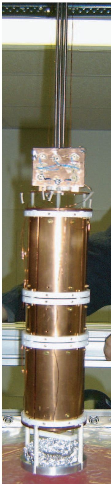
Figure 7-13: Cryogenic Preamplifier Mounted on the ICR cell
