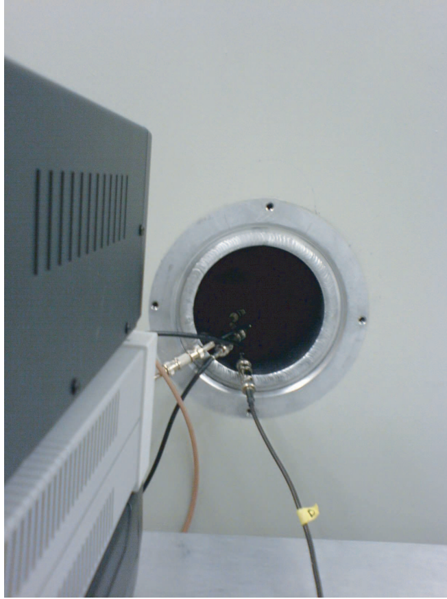
Figure 7-9: Preamplifier Inside the Bore of a Room Temperature 7 Tesla Magnet
