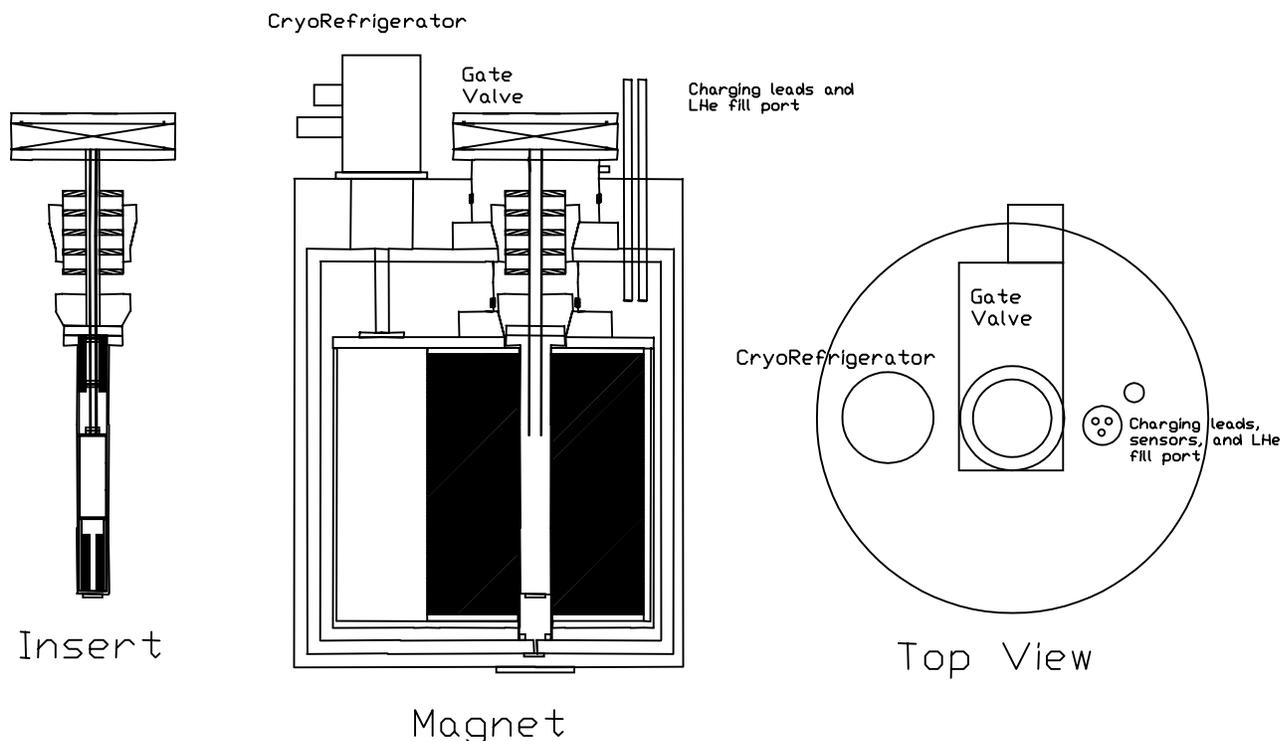
**Figure 1. Sketch of the Current CryoFTMS System Design**
